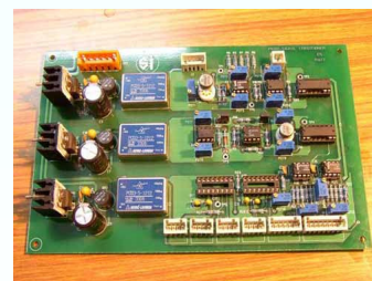
Three stage galvanic & two stage optical isolation signal conditioner
