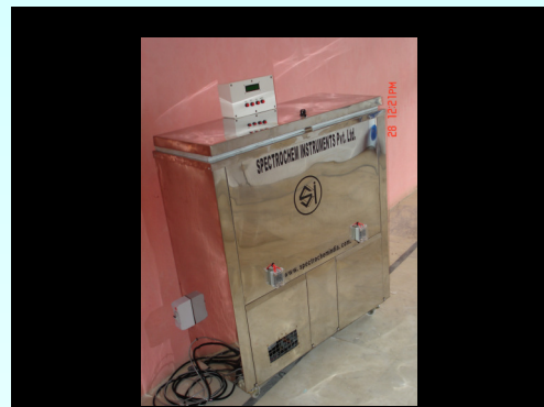
20L Hot, Cold & Tap water circulation system
